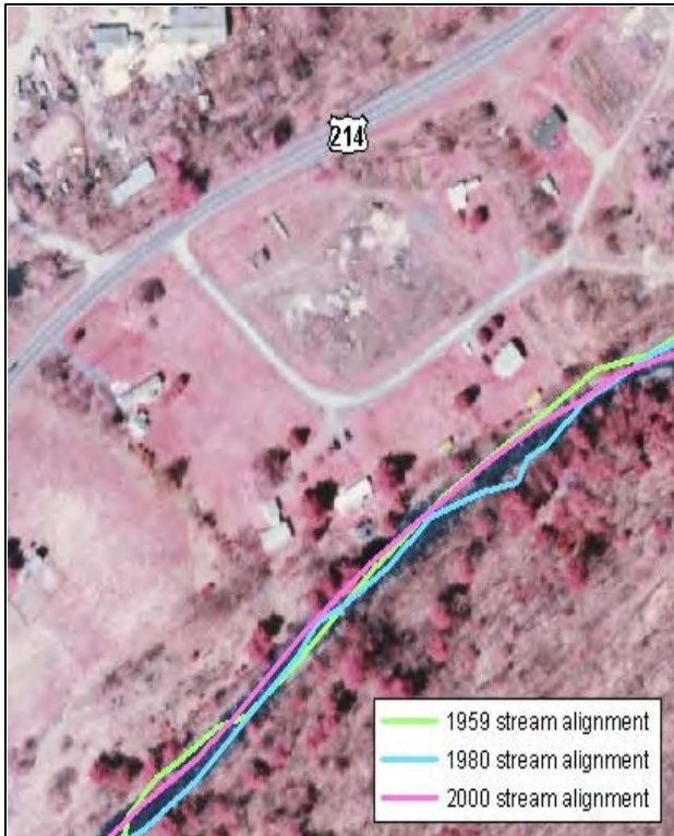
Figure 2 Historical stream channel alignments of Management Unit 9
