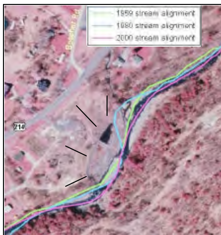
Figure 5 Historical stream channel alignments at bottom of Management Unit 8
