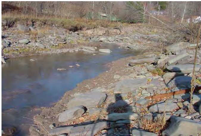
Figure 2: Coarse gravel/cobble materials seen on the right and left banks represent the channel invert elevation prior to downcutting. Note the clay present in the current channel bottom
