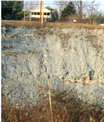
Looking at eroding bank with BEHI XS
