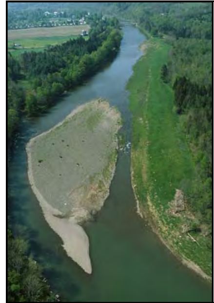
Figure III-14: Central bars indicate a loss of a stream's ability to transport sediment.
