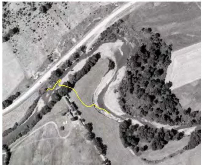
Figure VI-74: Close up of major meander shift in lower reach 4g. View of 1959 aerial photog with 2000 left bank location superimposed as yellow line. .
