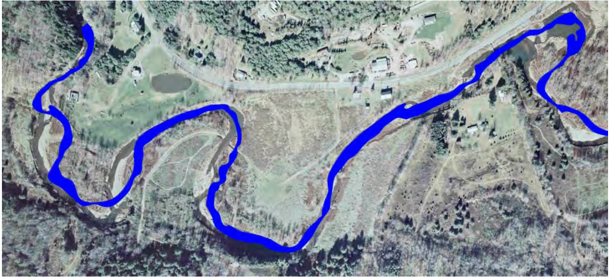
Figure VI-73: Aerial photo overlay of lower end of reach 4g showing 1959 stream channel (blue) superimposed over the 2000 photograph. Note significant meander shift in upper right corner along NYS Route 23.
